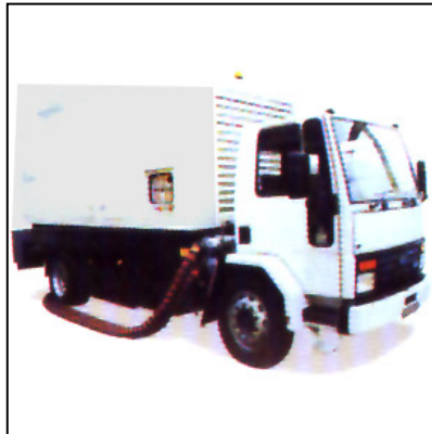
Air Start Unit
