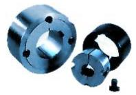
Adapter for taper bushing are recommended for use where it is moved convenient to straight bore than to drill,tap and taper bore hubs to accommodate bushings. The adapter is a taperbored sleeve with grey cast iron which fits into the straight bore of the hub. The bushing simply fits inside the adapter tightening the locking screws, adapter is expanded against the hub bore pressing the bushing tightly upon the shaft.
