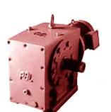
Wiperdrive helical-Bevel Geared motors and reducers are compact and highly efficient units, which are comparable with helical gear units. First stage reduction is by helical gear, a secondary spiral bevel gear set and third stage by helical hear.
